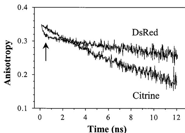
**Fig. 6.** Time-resolved fluorescence anisotropy of dsRed and Citrine (pH 9.0) by using TCSPC. The anisotropy of 490-nm excited Citrine decays as a single exponential with rotational time  $\phi = 16 \pm 2$  ns. To the contrary, dsRed anisotropy decays as a biexponential under the same experimental conditions, with a fast  $\phi_f = 211$  ps (indicated by  $\uparrow$ ) and a slow  $\phi_s = 53 \pm 8$  ns rotational time with fast-to-slow amplitude ratio of  $\approx 0.13$ .
