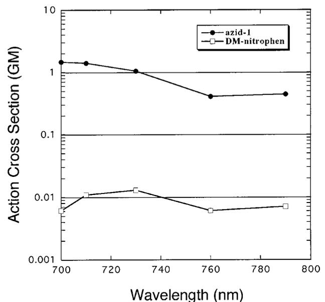
FIGURE 5 The two-photon uncaging action cross sections of azid-1 and DM-nitrophen between 700 and 800 nm expressed in GM, where  $1 \text{ GM} = 10^{-50} \text{ cm}^4 \text{ s photon}^{-1}$ . The values of the measured action cross sections are certain to within a factor of 2. NP-EGTA did not produce enough calcium for a reproducible uncaging signal to be detected above background noise at any of the wavelengths studied.
